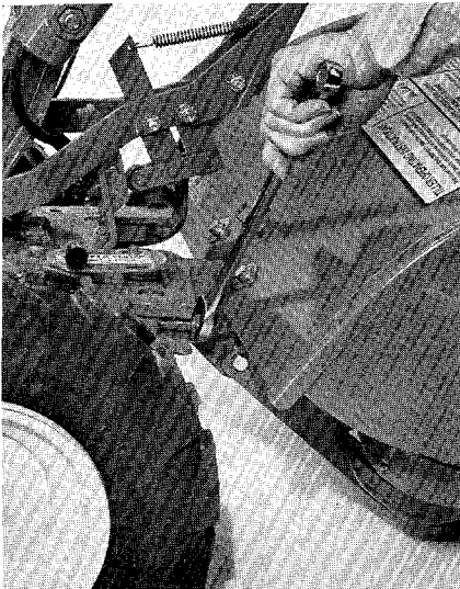
5-9: Tighten both swing-bolts.
